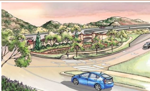
Rendering from EA illustrating pedestrian underpass in area planned for water quality treatment. Landscaping shown is schematic in nature as landscaping design will be completed by the City at a later date. Terraced wall, trail, and pedestrian underpass are included in the Build Alternative.
